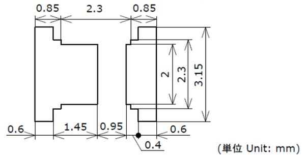
Figure 1. Recommended soldering pad pattern and recommended metal solder stencil aperture (example: part number NFSW757H-V1 Specification)
