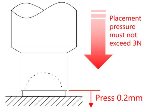
Figure 18. Nozzle Placement Depth
