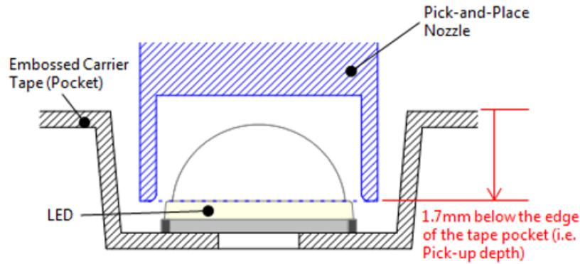
Figure 7. Recommended nozzle height (example: part number NFxW585AR Assembly Precaution application note)
