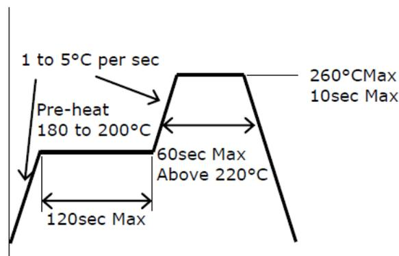
Figure 19. Recommended Reflow Soldering Condition (example: part number NFSW757H-V1 Specification)
