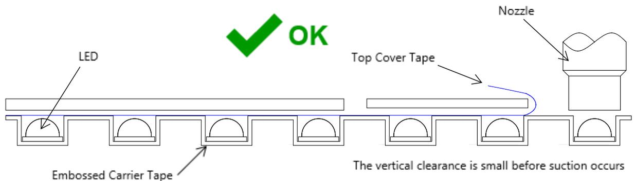
Figure 16. Removing the top cover tape just before suction
