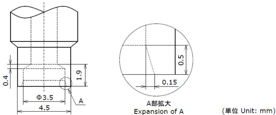
Figure 4. Recommended nozzle shape (example: part number NVSW119F-V1 Specification)
