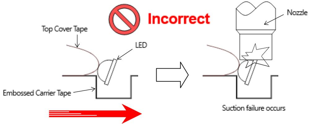
Figure 13. When the tape feeder feed rate is fast and the LED sticks to top cover tape
