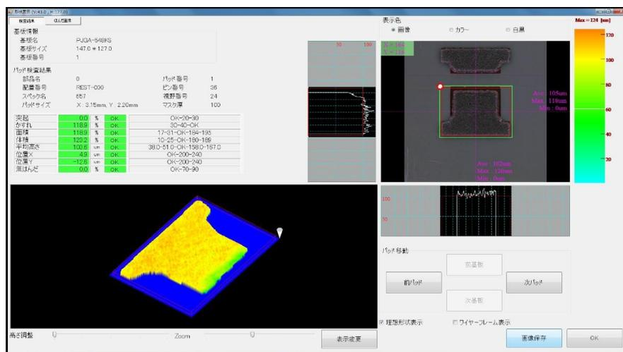
Figure 3. Example of the data for a visual inspection after solder printing
