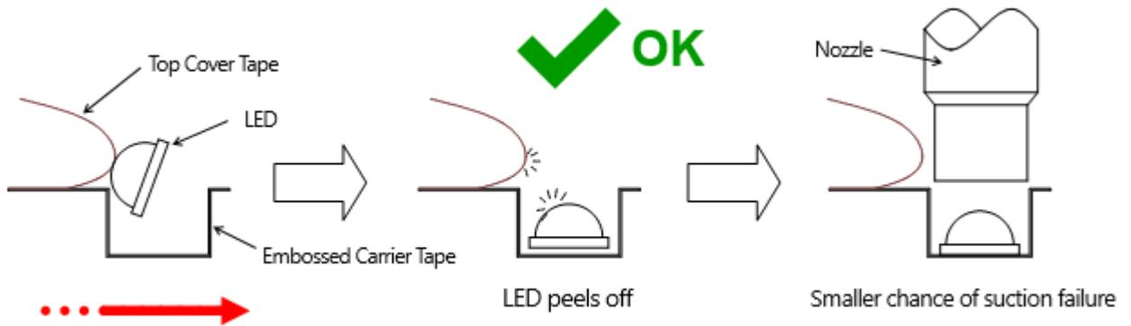
Figure 14. When the tape feeder feed rate is slow and the LED sticks to top cover tape
