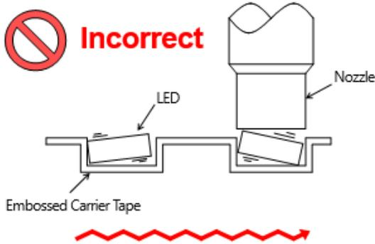
Figure 9. Tape feeder with large vibration
