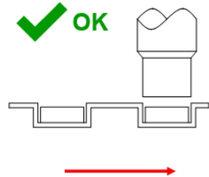
Figure 10. Tape feeder with small vibration
